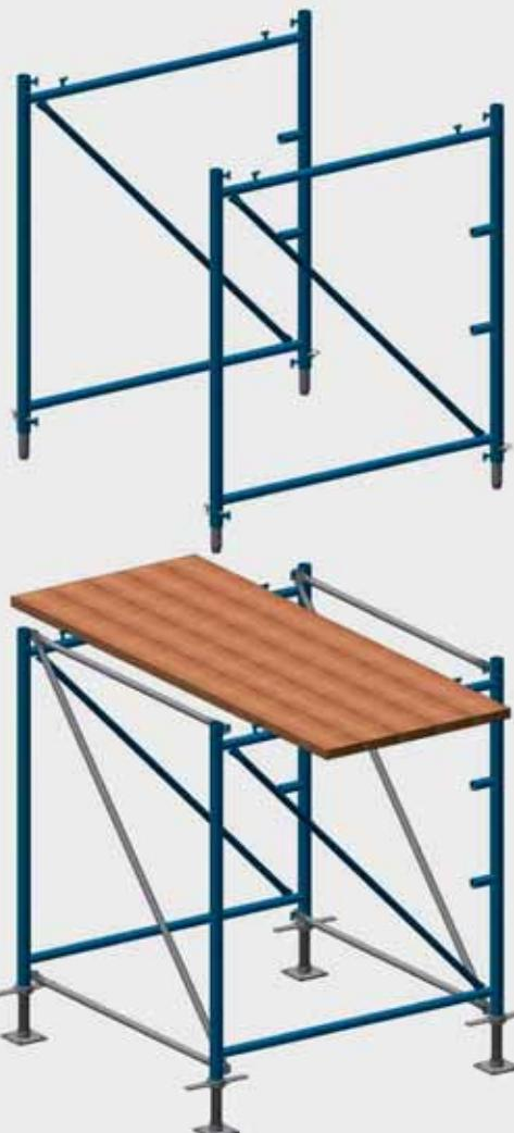
Assembled the first Tower's module, by the help of walking boards positioned on system frames, a working plan will be available in order to proceed with the repetition of steps for the foreseen levels of Frames
