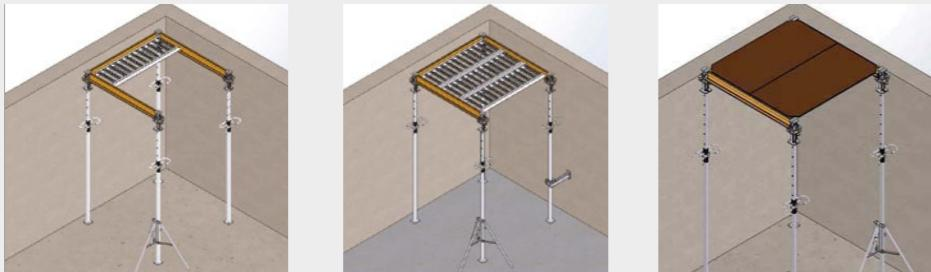
In order to ensure the system stability and lay-out positioning, other than the Tripods, the Wall Anchoring have to be used, anchoring the system, through the its Props, to existing structures. This done, as last in sequence, start to lay the System Grid or Alu Panels modules on top of the Alu Beams.
